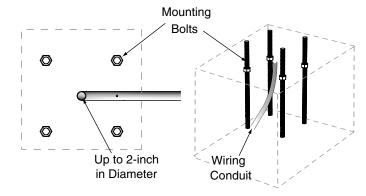
Figure 1 Mounting Bolts & Wiring Conduit Location
